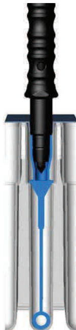
This illustration shows the three easy and rapid steps used to extract a sterilized 10uL Astral Loop from its sealed chamber.
