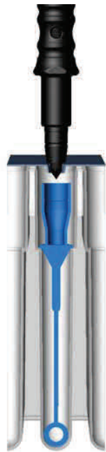
This illustration shows the three easy and rapid steps used to extract a sterilized 10uL Astral Loop from its sealed chamber.
