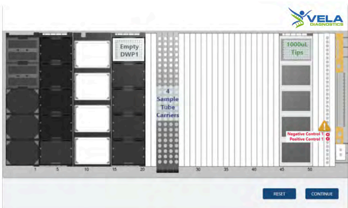
Figure 1. Layout of the Hamilton Microlab ® STAR ™ platform for 1 deepwell plate (1x96 tests) for sample plate preparation (refer to Appendix for 2 to 4 deepwell plates layout).
