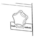
8. Once the scale column has been locked in place you may open the scale ramp as shown. The scale can also be used with the ramp in the closed position.
