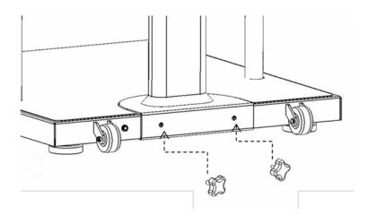
5. Attach the handles one at a time to the main column by inserting the bottom of the handle pole into the base and insert screw. Make sure to tighten screws to safely secure the handles to the base.
