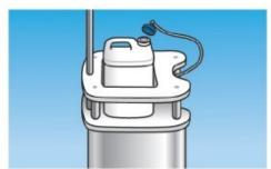
Connect Clorox Commercial Solutions® Clorox® Total 360® Disinfectant Cleaner<sub>1</sub> bottle to Clorox® Total 360® Electrostatic Sprayer. Put on appropriate PPE.\*
