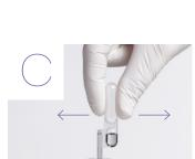
Release the upper bulb **slowly** to fill the shaft. **Keep** pipette tip submerged until shaft is full. Extra fluid should enter the lower bulb.
