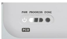
B. Check that the first progress indicator light is blinking. Lights will initially blink and then become stable as the test progresses.
