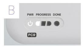
Check that the first progress indicator light **is blinking**. Lights will initially blink and then become stable as the test progresses. Note: If something different happens to the lights, please refer to the Troubleshooting Section.
