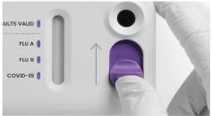
A. Slide the switch upwards in a firm, swift motion to close the sample port to start the test. Do not move test while running. Note: Make sure the switch is pushed all the way up.
