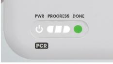
**D.** Wait approximately **30 minutes** for a green light to appear indicating the test is finished running.
