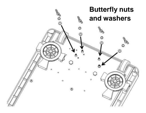
Step 3. Turn over the base and column and insert 4 washers, 4 lock washers and 4 butterfly nuts to attach the column to the base. Please make sure to tighten the 4 butterfly nuts to secure the column.
