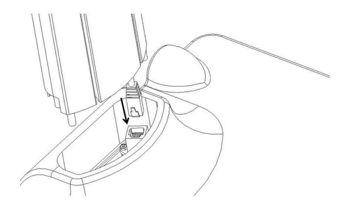
Step 1. Connect the cable to the base. The cable will be located inside the column.
