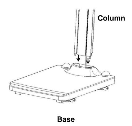
Step 2. Insert column into base as shown.
