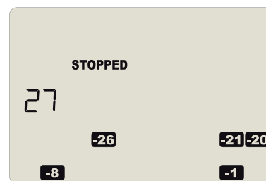
Figure 7: TRED30-16R stopped, showing '27' days of data has been collected.
