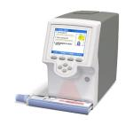
7 When the assay run is complete, remove and discard the assay tube.
